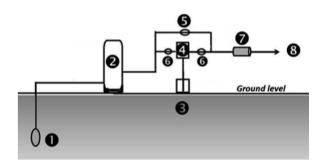
**Fig. 1.** Schematic view of the farm's water distribution system. 1: Borehole pump, 2: water buffering tank, 3: Dinastim<sup>™</sup> or Pigfast<sup>™</sup> delivery tank, 4: dosing distribution pump, 5: bypass, 6: pumps, 7: position of experimental coupons, and 8: to the troughs.
